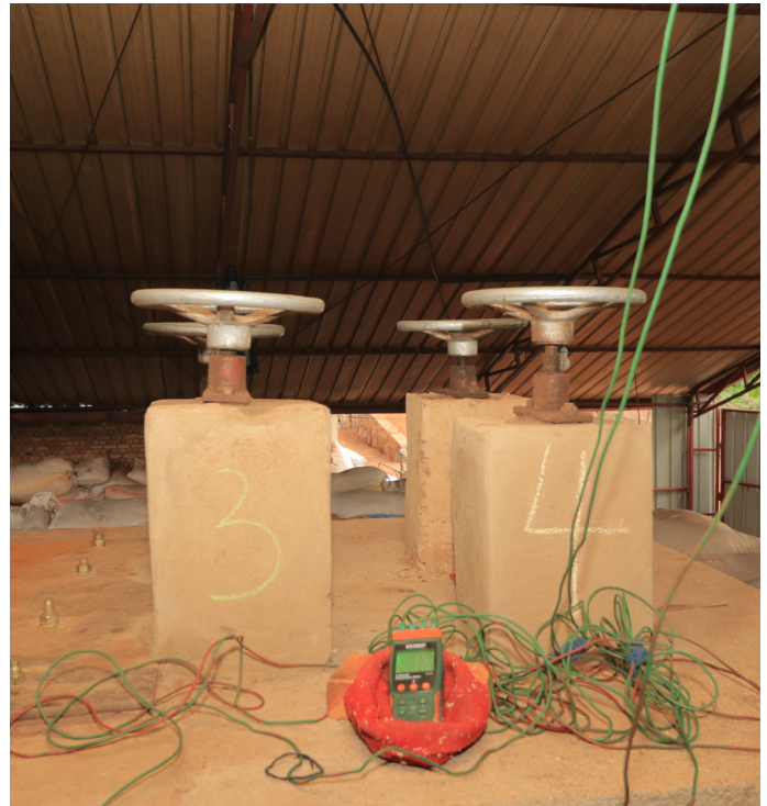
Zigzag kiln valves
