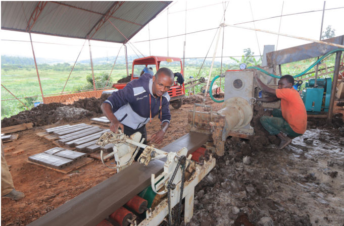
Slug Cutter aka Primary Cutter
