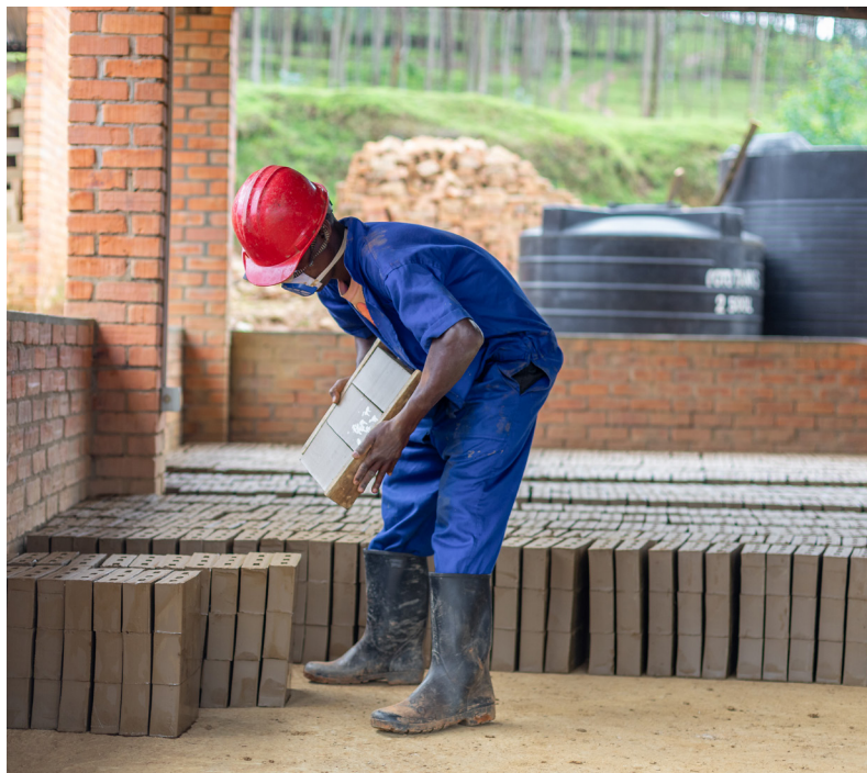
Direct handling from the cutting table
