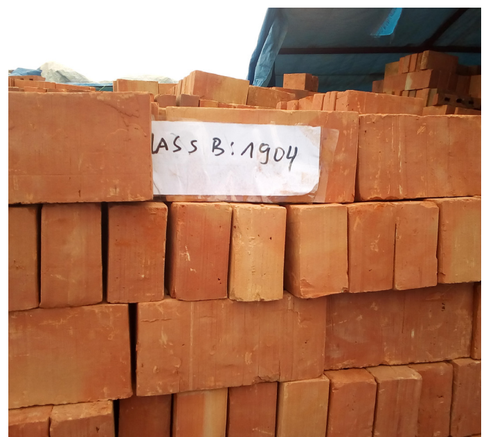
Bricks sorting after firing
