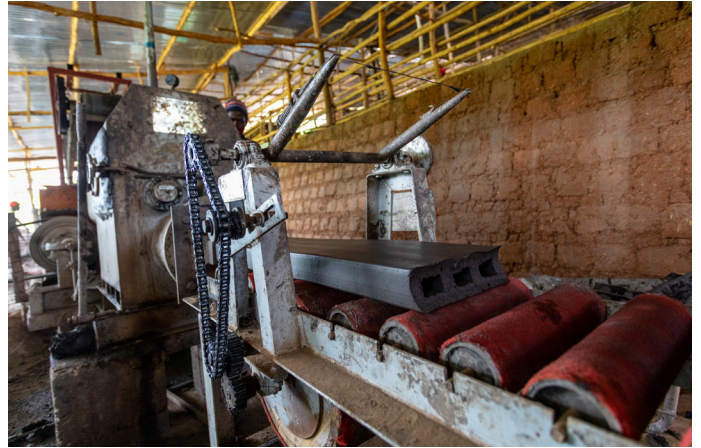
Brick column during extrusions and moulding
