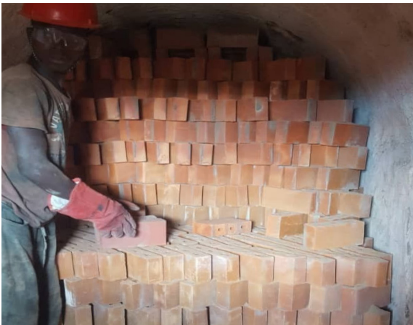
Kiln unloading
