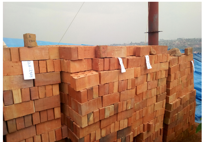
Bricks sorting after firing
